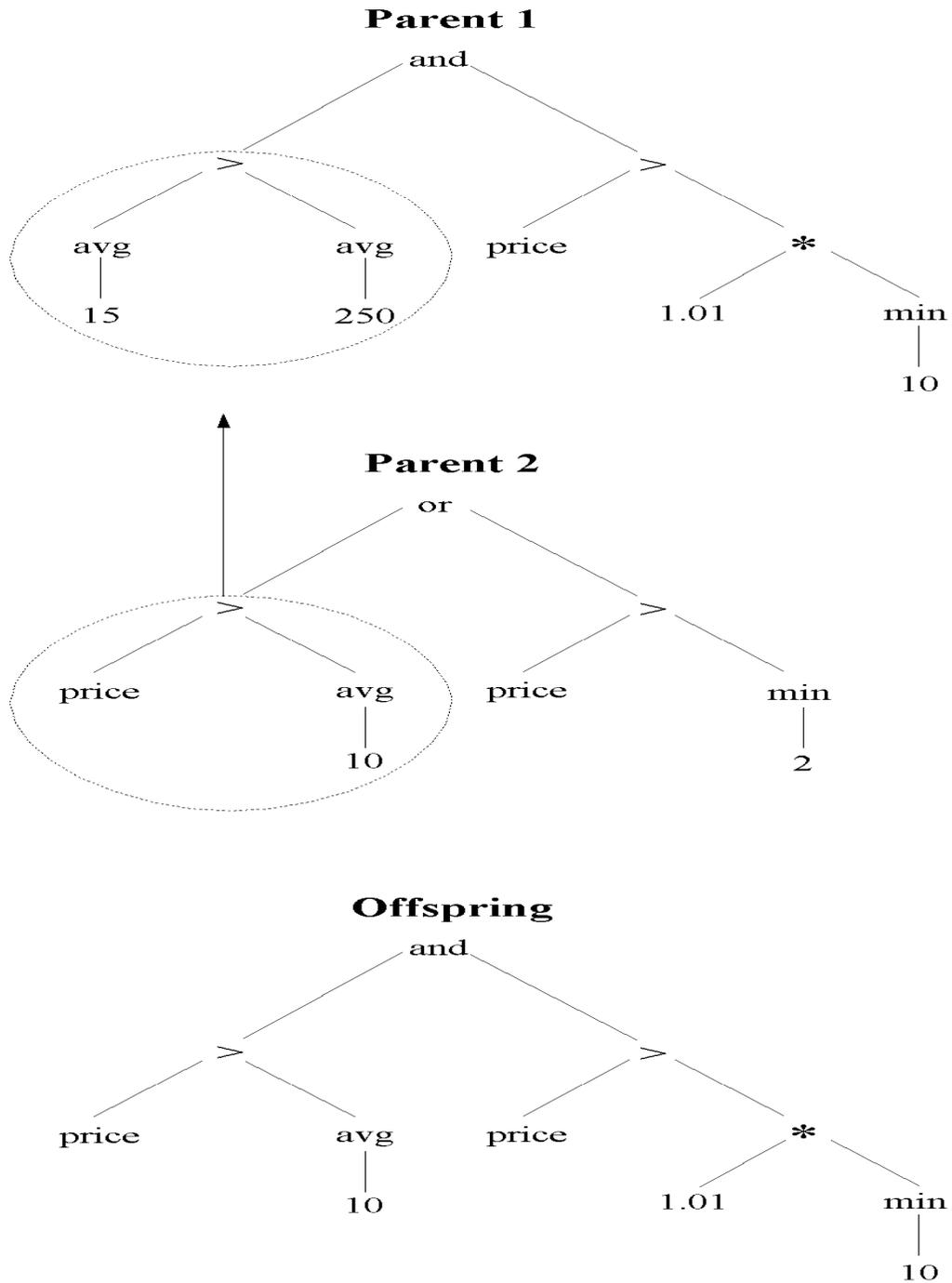
The recombination operation involves selecting random subtrees from each parent rule, and replacing one with the other to create a new rule, labeled "offspring".
